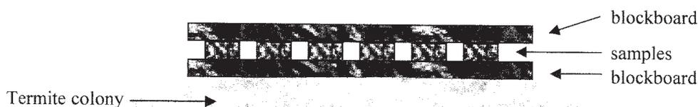
Figure 1. Subterranean termite resistance test of the composite board in the field
