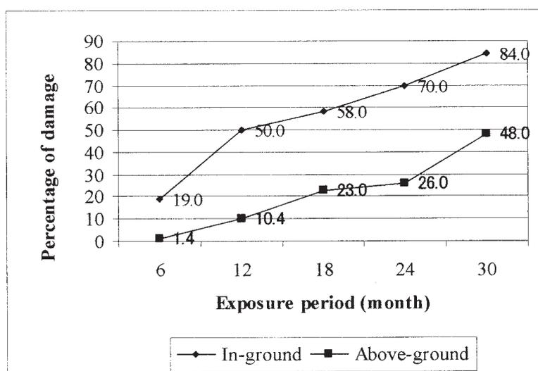
**Figure 2.** Average percentage of damage of untreated roundwoods (control) in “in-ground” and “above-ground” conditions.
