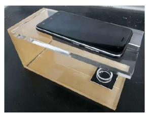
**Figure 1.** Photography devices. Termites were placed in the ring. Cellular phone was placed on an acrylic stage with its lens aiming at the termite through the gap.
