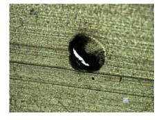
Figure 8. Termite nibbling on barrier A
