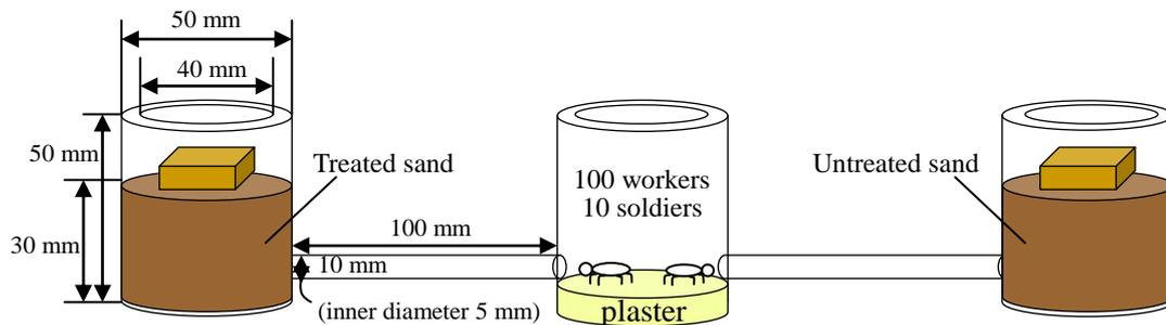
Fig.2. Experimental device of soil choice-test for *C. formosanus*
