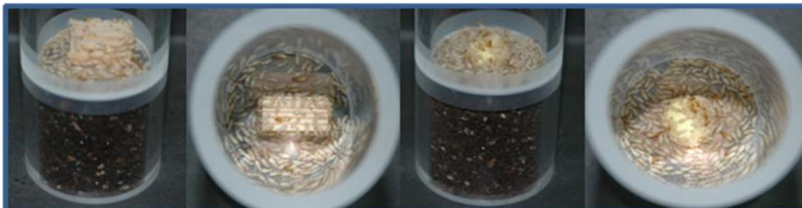
Fig. 1 Test method (G) using 300 workers and 30 soldiers of *Coptotermes formosanus* with a sugi wood block (1 x 1 x 2 cm) and a pine wood block (3 x 3 x 0.5 cm) in the upper and lower-chambers, respectively [ (1) and (2)] or a small amount of plaster [(3) and (4)] in the upper chamber instead of sugi wood block
