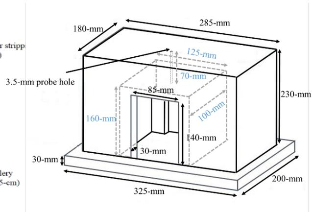
Fig. 2 The polystyrene foam test chamber
