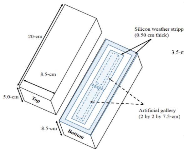
Fig. 1 The sandwiched sample
